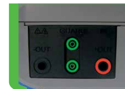
Guard terminal for connecting shielded test leads
