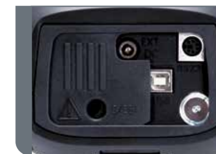
USB and PS/2 connectors for communication with PC and barcode scanner.
